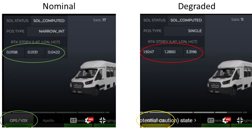
Figure 19. GPS data showing nominal and degraded RTK performance
