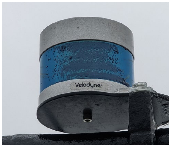
Figure 37. Obscured lidar located on the top of the AV
