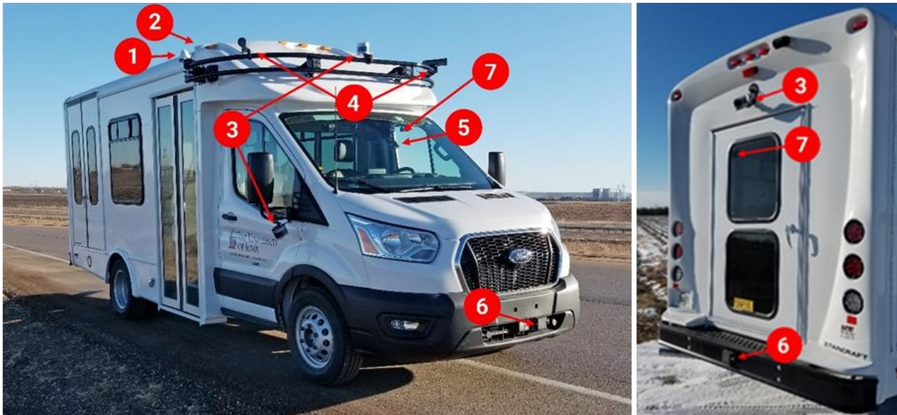
Figure 12. Location and description of sensors (LiDARs, radars, and cameras) and other instrumentation
