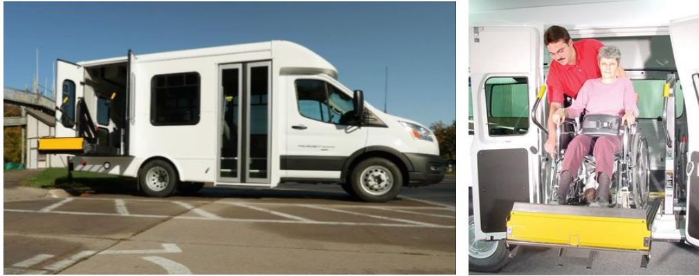
Figure 4. Passenger side view with ADA compliant entry door and wheelchair lift (left) and passenger being unloaded using wheelchair lift (right)
